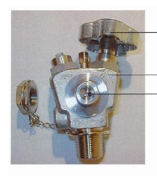
Hanwheel on the Liquid spindle
